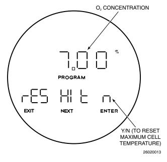
Figure 3-12. RESET MAX CELL T
